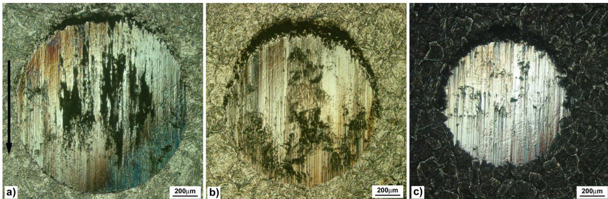
Figure 4, Wear craters of plasma nitrided SMSS samples at (a) 400°C, (b) 450°C and (c) 500°C after 5min (200m) of testing.
