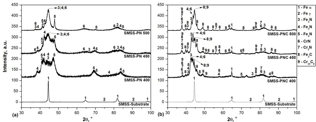
Figure 2, X-ray diffraction patterns of plasma (a) nitrided and (b) nitrocarburized SMSS samples at 400, 450 and 500°C.
