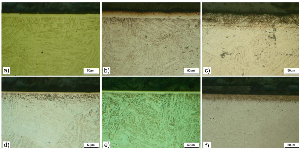
Figure 1, Optical cross sections of plasma (a-c) nitrided and (d-f) nitrocarburized SMSS samples at (a, d) 400°C, (b, e) 450°C and (c, f) 500°C.
