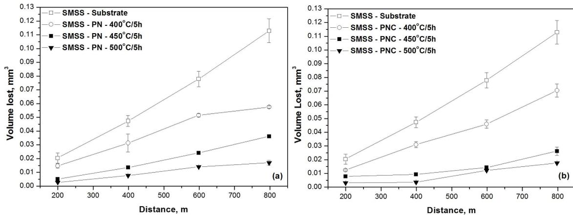
Figure 3, Wear volume loss curves of plasma (a) nitrided and (b) nitrocarburized SMSS samples.
