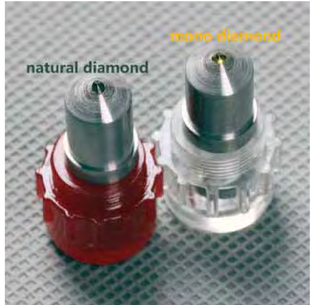
diamond spheroconical indenter 120°; 0.2mm radius of curvature (Brale indenter)
