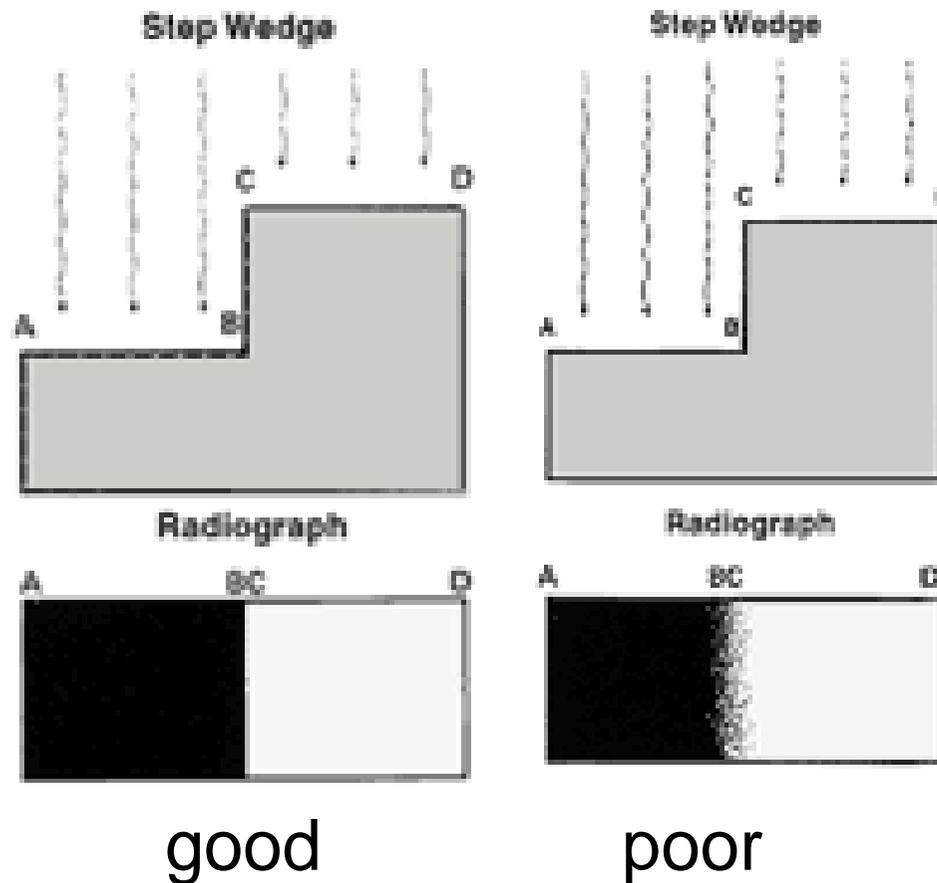
**High definition:** the detail portrayed in the radiograph is equivalent to physical change present in the part. Hence, the imaging system produced a faithful visual reproduction.
