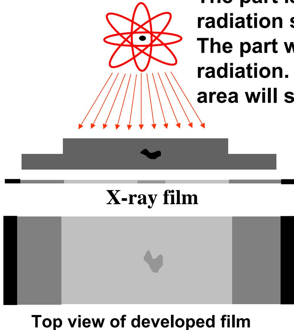
The part is placed between the radiation source and a piece of film. The part will stop some of the radiation. Thicker and more dense area will stop more of the radiation.
